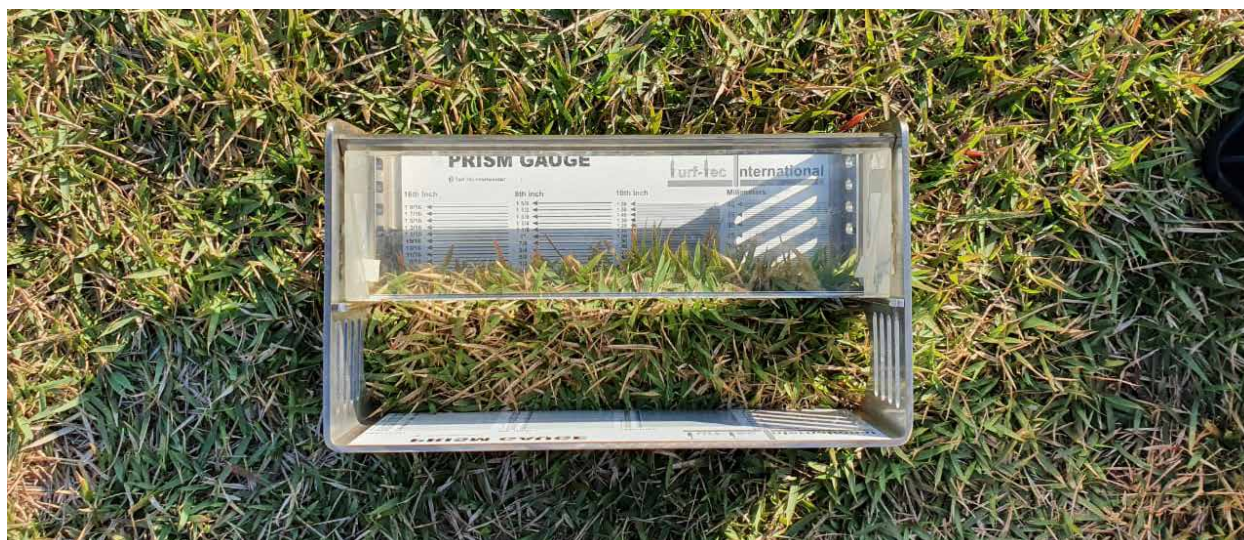
Figure 4. Measurement of Esmeralda zoysiagrass height using a Grass Height Prism Gauge.
