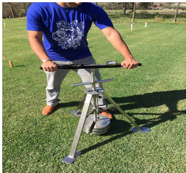
Figure 5. Turf traction resistance testing with the Rotational Resistance Tester – Deltec Metaal®.
