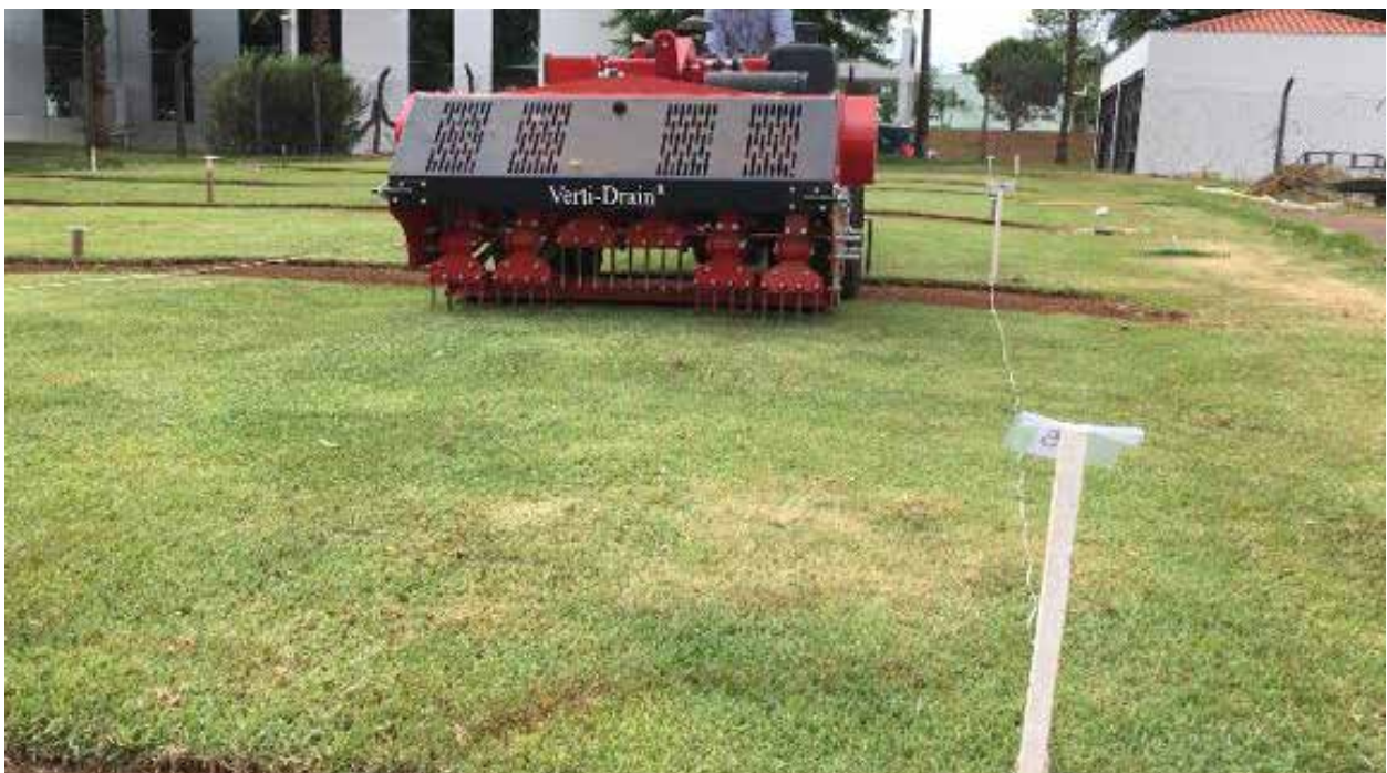
Figure 3. Soil aeration using Verti-Drain® in the Esmeralda turf experimental area.
